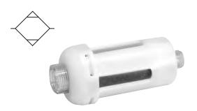
Used at the point-of-use, this disposable, mini inline desiccant dryer removes all traces of water vapor, oil vapor and dirt. It is often used directly upstream of blow guns or spray guns as final protection for critical parts blow off and paint spraying. Install in either direction; it functions in both directions.
